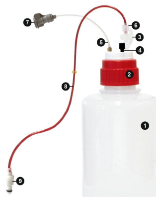
Figure 2. PPCO bottle assembly. (1) PPCO bottle, (2) B53 cap with PTFE inlay with three ¼"-28 UNF ports, (3) 2-way Luer stopcock, (4) PP plug, (5) 1/8" OD FEP mobile phase suction line, (6) 1/8" OD tubing Luer connector, (7) quick connector mobile phase line, (8) 1/8" OD PU inert gas supply line, (9) quick connector inert gas line.
