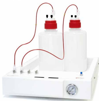
Figure 1: ET 210 eluent tray - Saving inert gas by blanketing: The ET 210 has 4 valved gas outlets facilitating up to 4 mobile phase bottles, which can be independently kept under inert gas atmosphere (blanketing).
